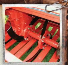
The Verti-Quake is a rotary aerator that decompacts the soil using a set of rotating steel blades. As these blades cut cleanly through the soil, they create a wave action that shatters compacted areas and opens up the subsoil.The Verti-Quake is available in two different models and can work at depths up to 10" with little or no surface disruption.
